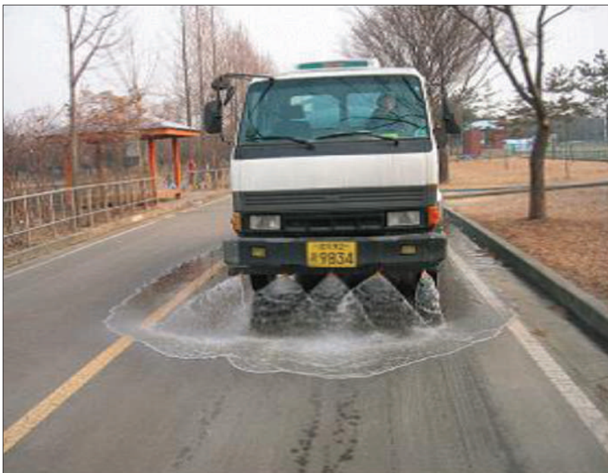
Figure 7.18 Water from Jungnang sewage treatment plant reused for road cleaning
