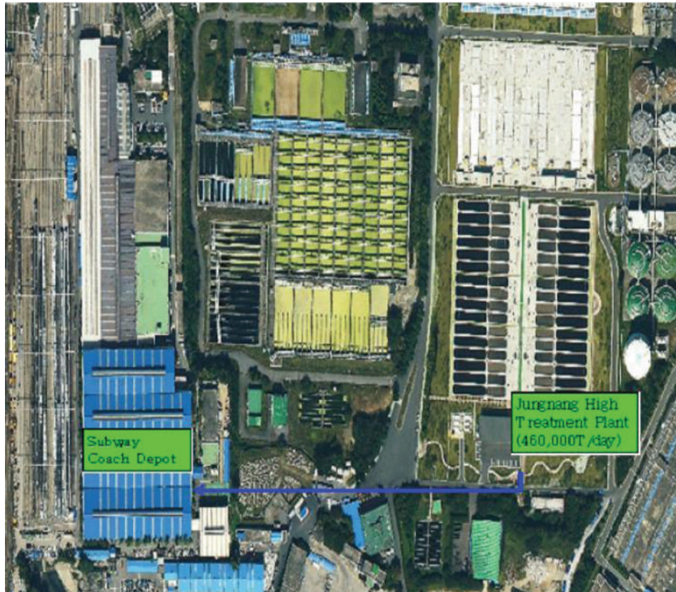
Figure 7.19 Highly treated sewage used at subway coach depot for cleaning
