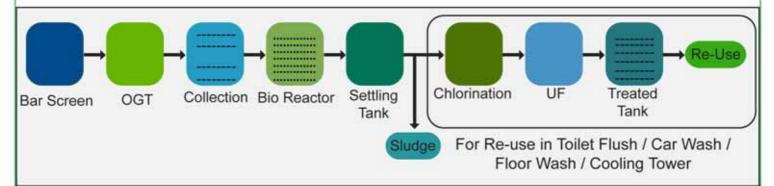
Sewage Treatment with advanced process for use of Treated Water for all Domestic needs.
