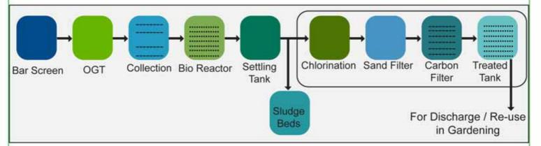
Sewage Treatment with advanced process for Re-use of Treated Water for High Quality Applications
